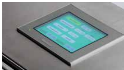
PLC-Software with HMI touch panel
